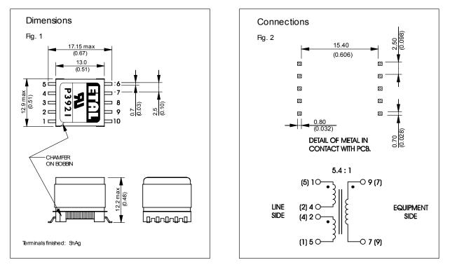
Dimensions shown are in millimetres (inches). Terminal references in parentheses denote alternative customer designation.
